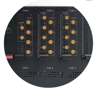
In FXE phase difference mode between channels, the fluctuations of the common LO cancel out, thus allowing for very high quality phase comparison between highly stable clocks like H-Masers, even with only moderate requirements for the stability of the common local oscillator.
